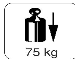
$$D = \frac{\text{MAX KG} \times \text{MAX KG}}{\text{MAX KG} + \text{MAX KG}} \times 0,00981 \leq 7,52 \text{ kN}$$
