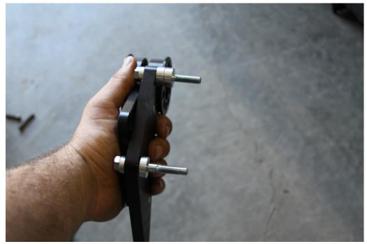
7. Place adjuster assembly into sled and thread bolts into the threaded bulk head.
