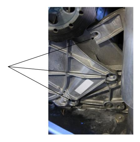
5. Insert new button head cap screw supplied with the kit from inside of the tunnel outward and place ¼ inch spacer on bolt. Pictured below
