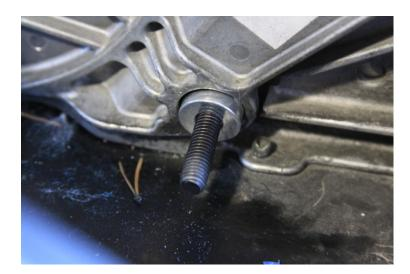
6. Place bolts with washers into the belt adjustment bracket, place 1 5/8 inch thick washers on the top bolt closest to the idler pulleys and 1, ¼ inch thick washer on the middle and bottom bolt. Place a small drop of blue loctite onto threads of bolts. See picture below
