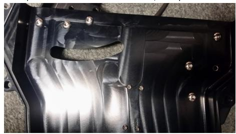
22. Now on the front of the cover use the 2 remaining stainless screws to plug the bottom 2 holes on the brackets. This is so the tank will not slide through the bracket. Make sure to use a drop of loctite on the threads.
