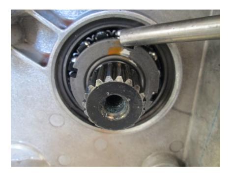
6. Place the provided piece of pipe over the end of the shaft so it securely comes in contact with the threaded sleeve.
