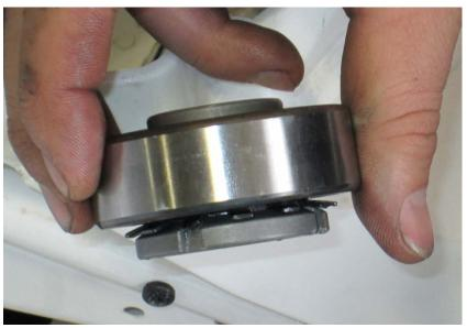
13. The case will need to be reheated so that the bearing will easily slide into the pocket in the chain case.
