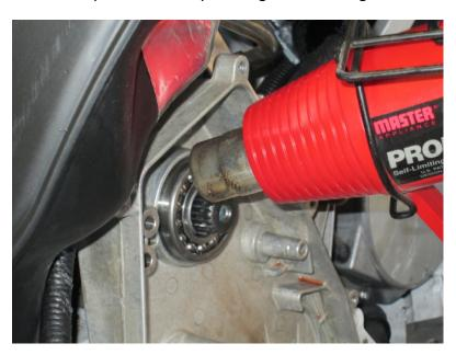
10. Use a couple screw drivers or picks to pry the bearing out. The case will be hot so proceed with caution.
