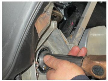
15. Once case has cooled you can tighten the top retaining nut, use the hammer and punch and rotate the nut clockwise.
