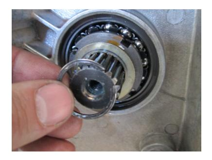
5. Using a hammer and punch bend the star washer tabs out of the slots on the retaining nut so that the nut can be removed. Use same hammer and punch and back the nut off counter clockwise.
